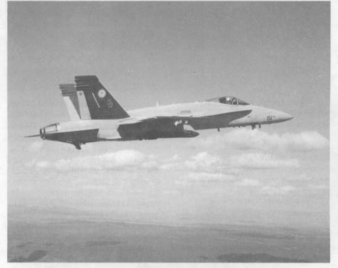
F-118 AIRCRAFT carries a B90 Nuclear Depth Strike Bomb during an in-flight test to check NDSB separation from the aircraft. (US Navy photo)
